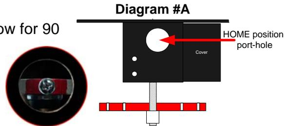
For 180 degree rotation, remove the limit screw currently in the home position and move it to the secondary porthole located opposite the drive motor.
