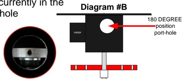
For 355 degree rotation simply remove the limit screw from the home position.
